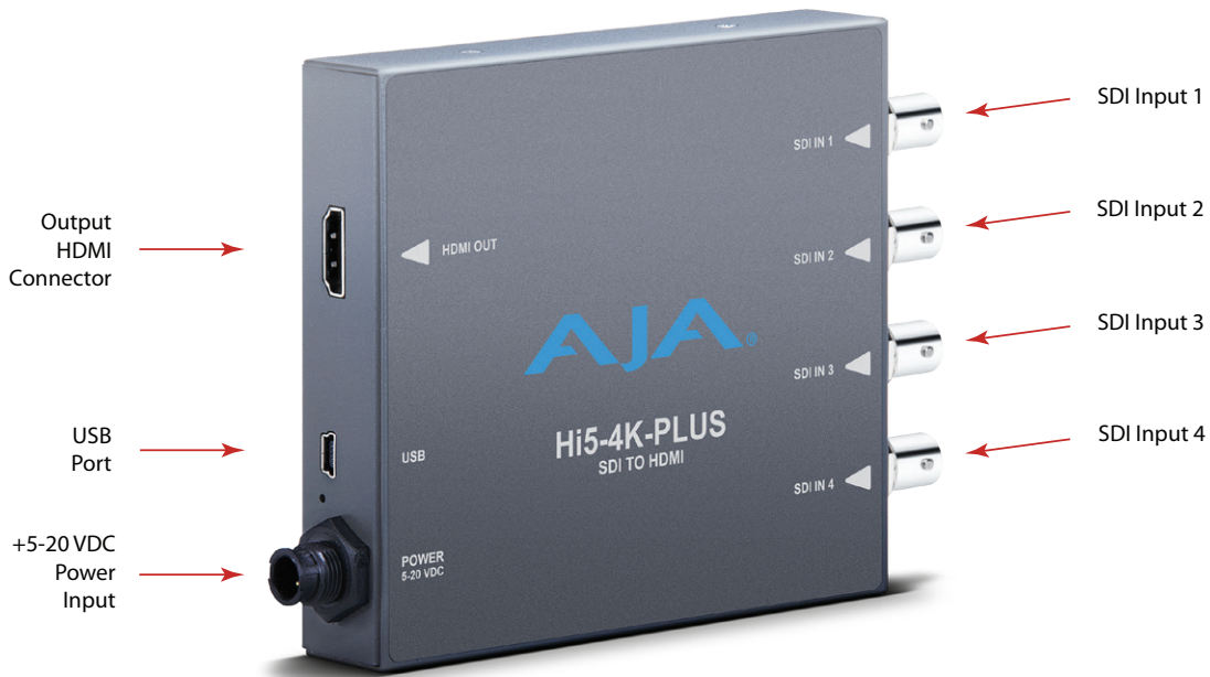
Figure 2. Hi5-4K-Plus Converter Connections
