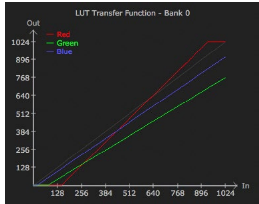
Figure 14. Example LUT Transfer Function Curves
