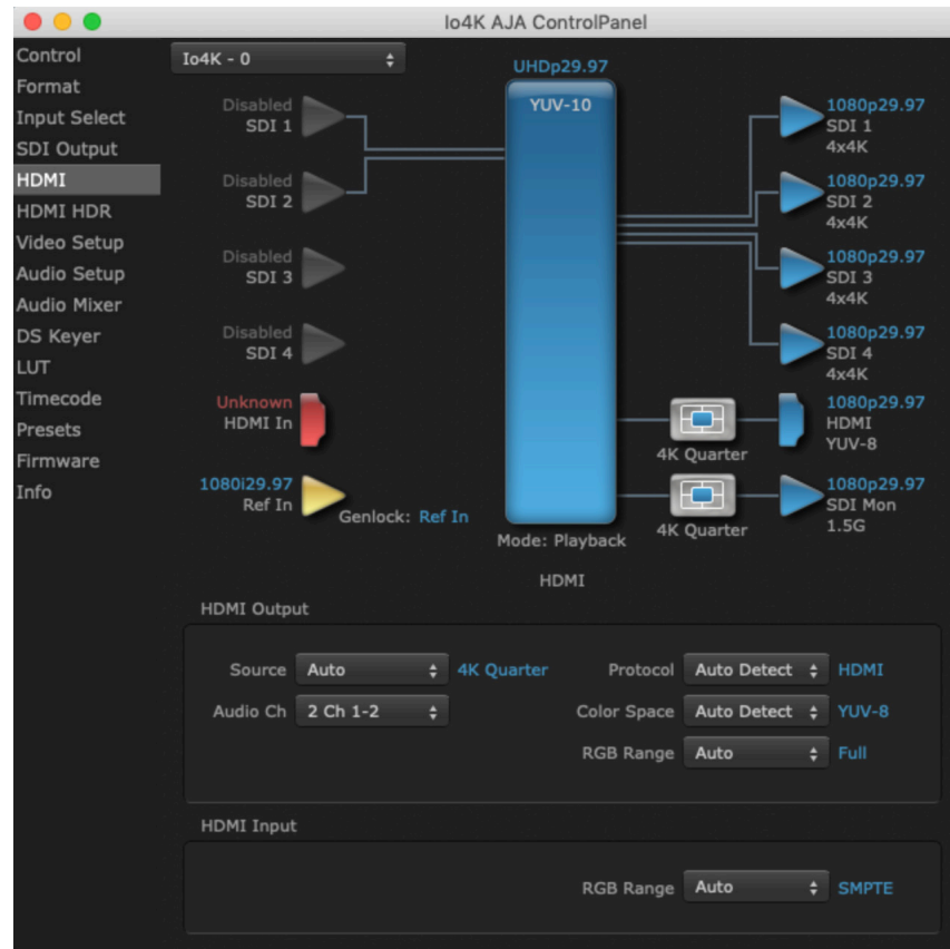
Figure 20. HDMI Output Screen with Quad HD Output Configuration
