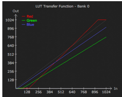
Figure 13. Example LUT Transfer Function Curves
