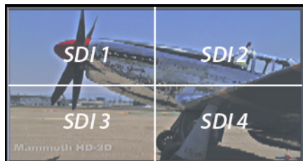
Figure 14. Mapping of Quad SDI Outputs
