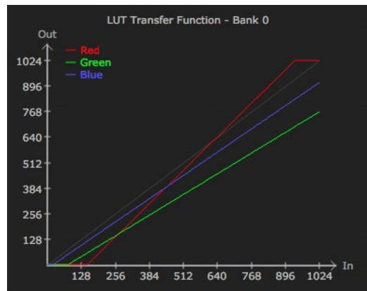
Figure 13. Example LUT Transfer Function Curves
