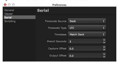
In the following procedure, you will use the Capture Offset for Capture timing and Output Offset for Edit-To-Tape. Offset values presented are in whole Frames and tenths.
