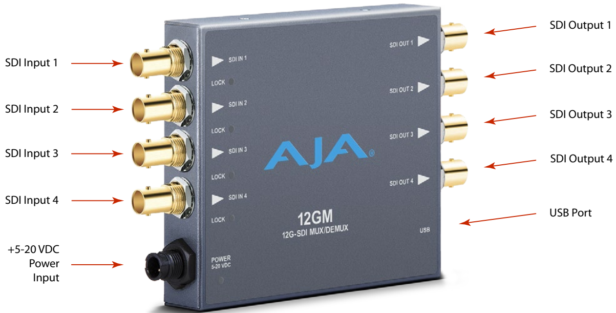
Figure 2. 12GM Converter Connections
