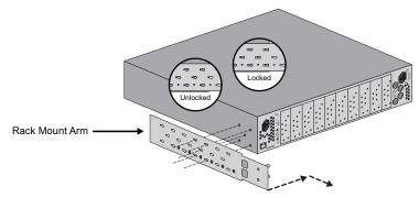
2. Install the Rail Guides for each Rack Mount Arm.
