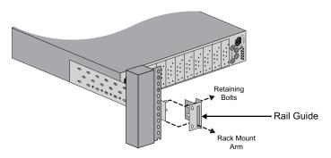
3. Secure the Rail Guides and Rack Mount Arms to the rack.
