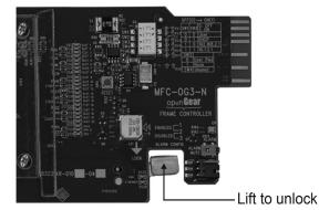
5. Insert the Network Controller Card, with the component side out into the card guides between the dividing wall and the last slot, ensuring the card does not touch the Card Retaining Screw.
