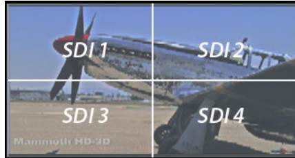
Figure 41. Mapping of Quad SDI Outputs
