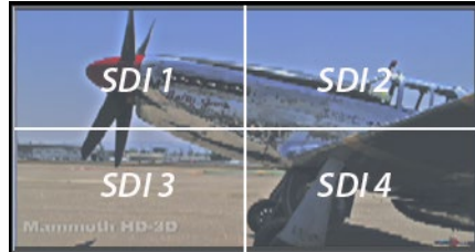
Figure 15. Mapping of Quad SDI Outputs
