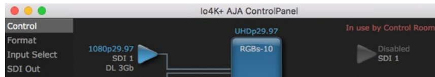
Figure 5. Control Panel In Use Message (in red)
