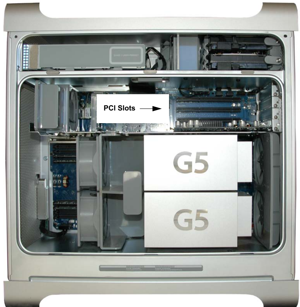
Locate the PCI Slots Inside Your PowerMac (G5 Shown Here)
