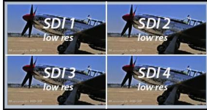
For 2SI UltraHD or 4K SDI video at 30 fps or less, monitoring one of these four signals on a standard SDI monitor displays the entire picture, but at a lower resolution. Above 30 fps, 3G bandwidth is required, so a 3G capable monitor is required.”
