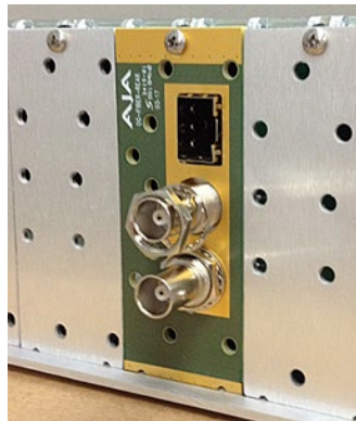
Figure 5. BNC Star Washer and Nut Installation
