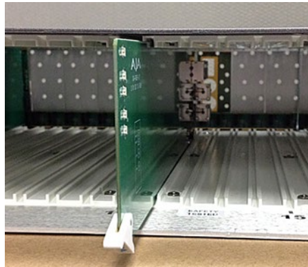
Figure 4. OG-FIBER Card Inserted Into Left Slot
