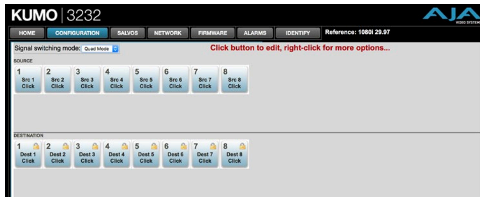
Figure 18. Quad Mode Reduced Sources and Destinations
