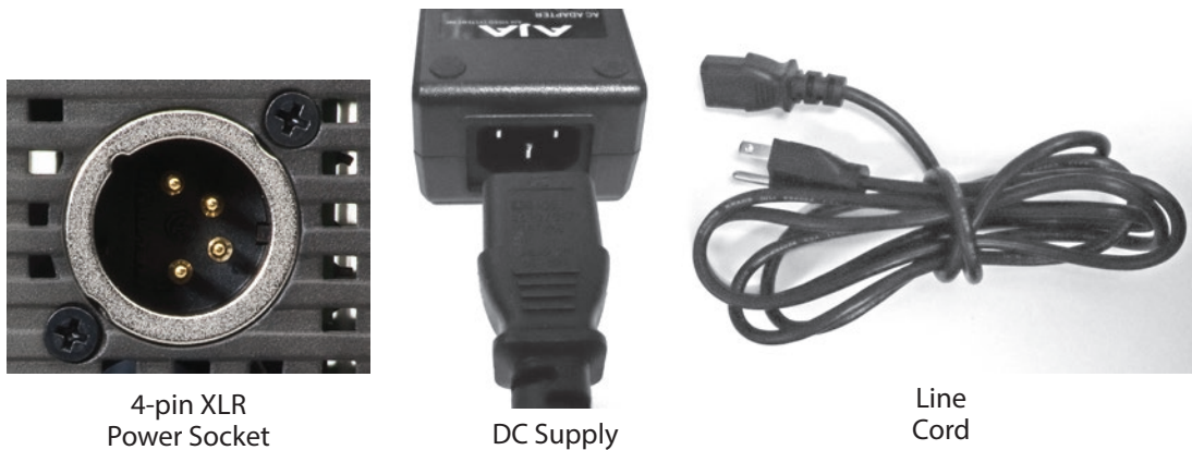
Figure 4. Ki Pro Ultra Plus Power Supply Connections
