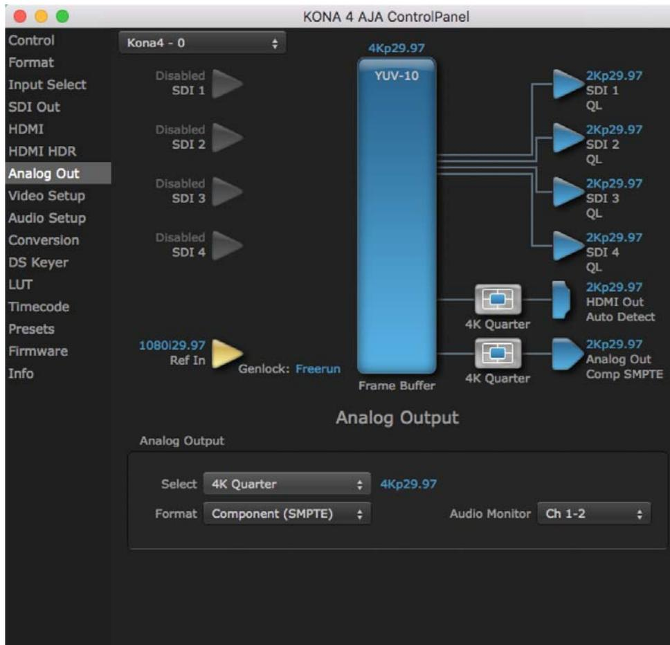
For 4K formats, a Quadrant Select menu is available to choose the desired quarter-segment of the 4K display for Analog Output to a monitor (see the discussion on 4K quadrant mapping at this beginning of this section).
