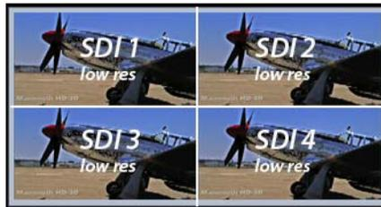
For 2SI UHD or 4K SDI video at 30 fps or less, monitoring one of these four signals on a standard SDI monitor displays the entire picture, but at a lower resolution. Above 30 fps, 3G bandwidth is required, so this type of signal cannot be monitored on a standard SDI monitor using only one connector.
