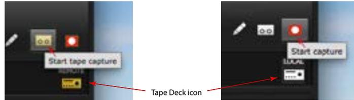
**NOTE:** If the Tape Deck icon is lit (yellow), AJA Control Room is detecting an RS-422 connection that is active. If it is white, there is no active RS422 connection.
