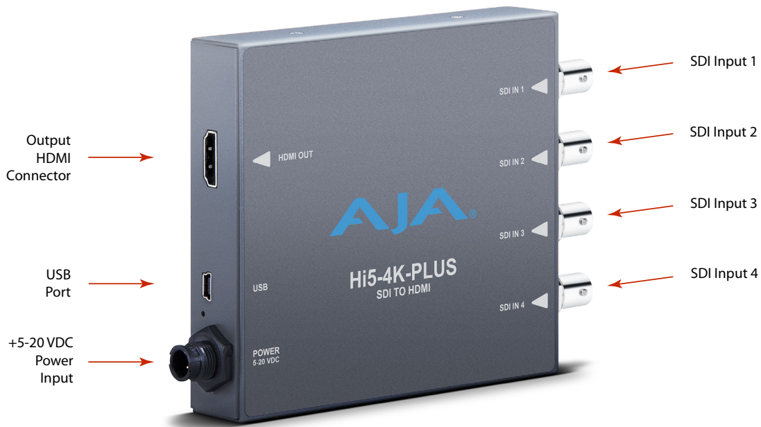
Figure 2. Hi5-4K-Plus Converter Connections
