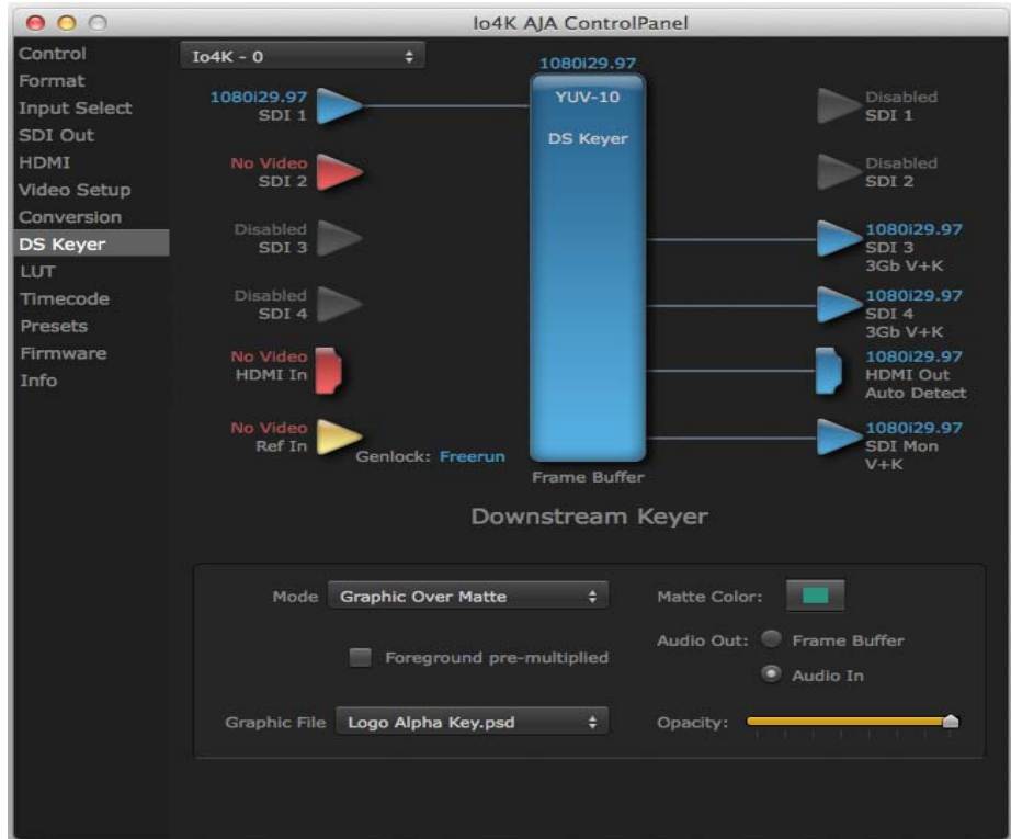
Figure 22. AJA Control Panel, Downstream Keyer Screen
