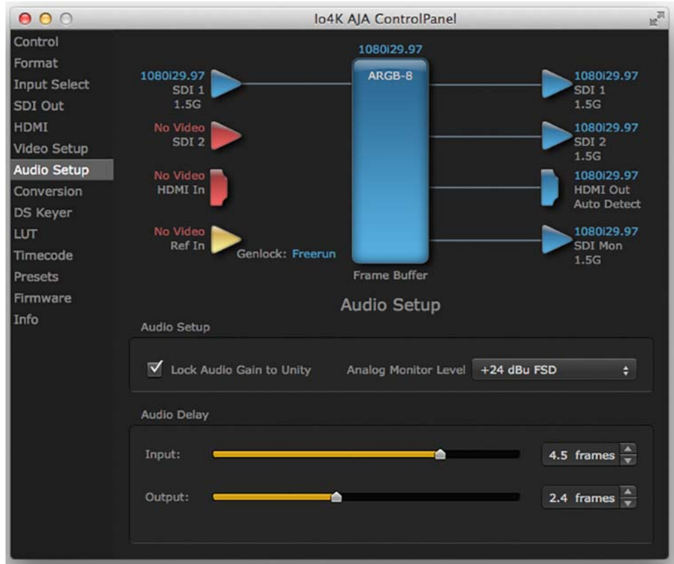
Figure 19. AJA Control Panel, Audio Setup Screen
