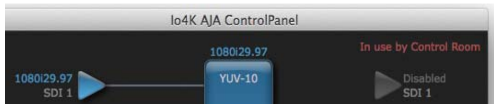
Figure 9. Control Panel In Use Message (in red)
