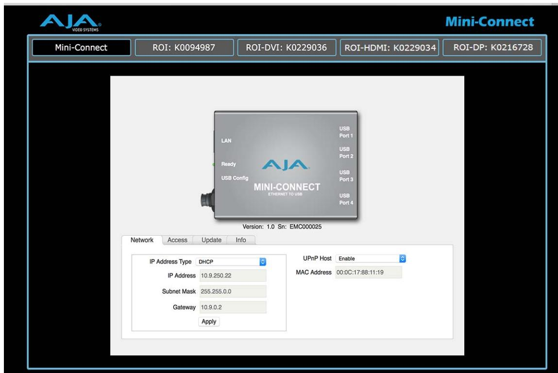
Displayed below the graphic image are the version of firmware currently installed in Mini-Connect, and the factory set unique serial number of your Mini-Connect. If you ever call AJA Support for service, you may be asked for this serial number.
