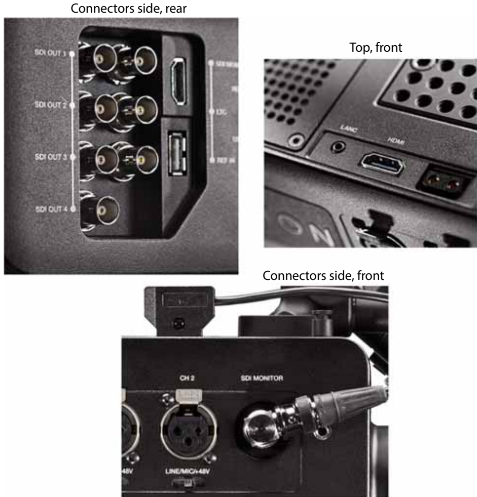
Figure 11. Front & Rear Video Connector
