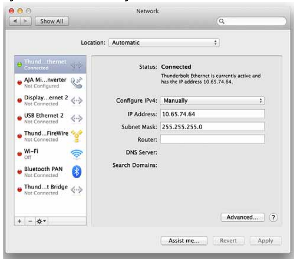
Figure 17. Default IP Address Configuration
