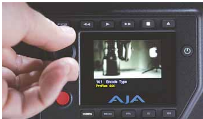
Figure 5. CION Onboard User-Interface Screen and Controls
