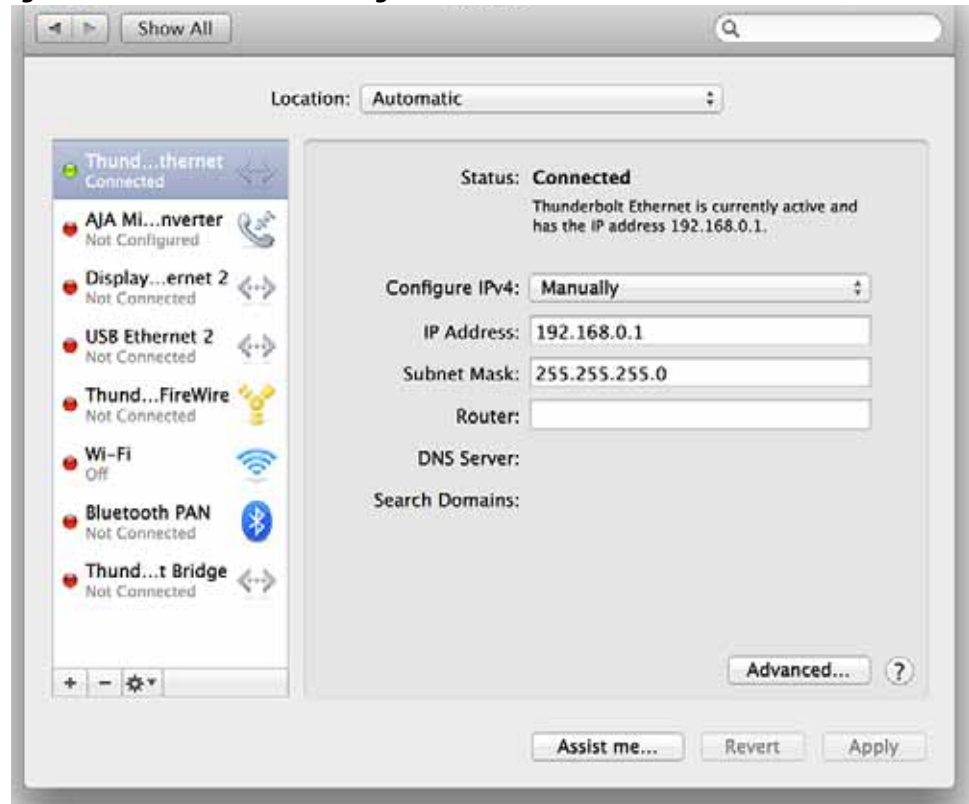
Figure 18. Static IP Address Configuration
