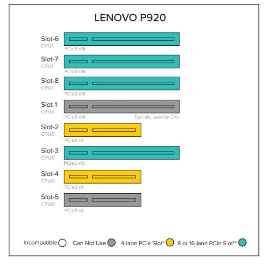
For high-demand workflows such as 4K I/O or above, it is recommended that the AJA Video I/O card or device be on a separate PCle bus from the media storage adapter.
