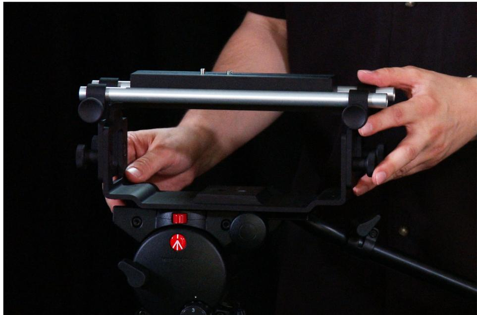
Remove the sliding plate from the top of the Exoskeleton by twisting the locking knob counterclockwise, then slide the plate free. Place the camera on the mount, orienting the mount's alignment pin to the camera's corresponding pin socket. Once aligned, tighten the mounting screw to secure the camera. Slide the camera and mount back on the rail and tighten the locking knob.
