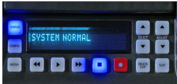
You can exit STATUS just as you can with the CONFIG and MEDIA buttons, by simply hitting the STATUS button again, or hitting the stop button.
