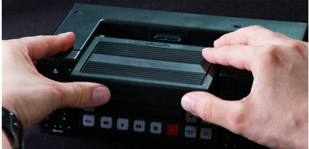
With the media inserted, position Ki Pro near the camera or mount Ki Pro to a camera with the optional Exoskeleton.
