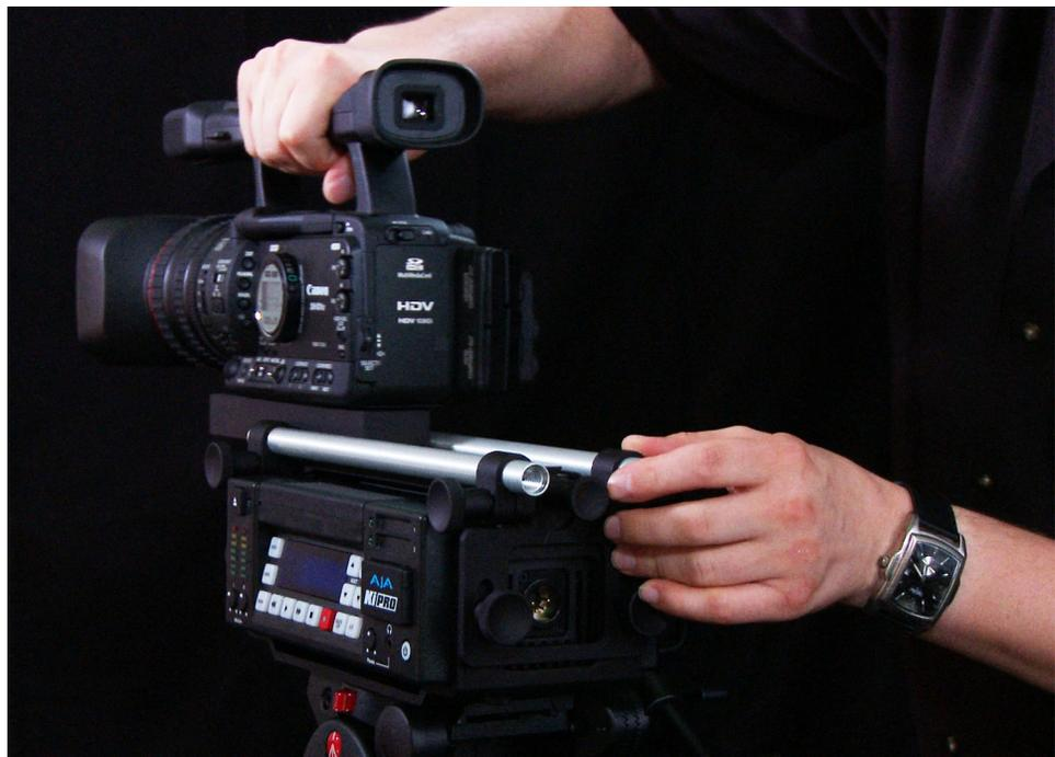
Slide Ki Pro into the Exoskeleton from the right hand side with the locking knob facing the rear. Center the 4-pin XLR power connector in the rear opening of the Exoskeleton. Anchor the Ki Pro in the Exoskeleton with the two thumbscrews.
