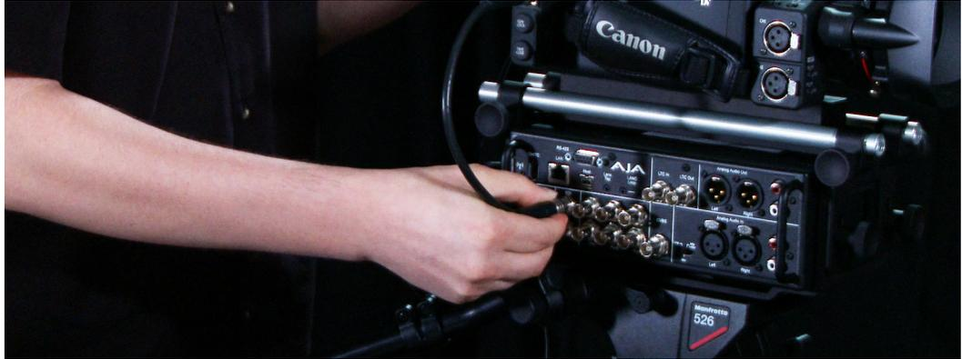
If you have a camcorder with an HDMI output, it can also provide audio and video - but not timecode - with one single cable to Ki Pro.
