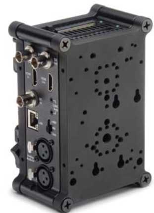
Example: Two mounting plates attached to a Ki Pro Mini
