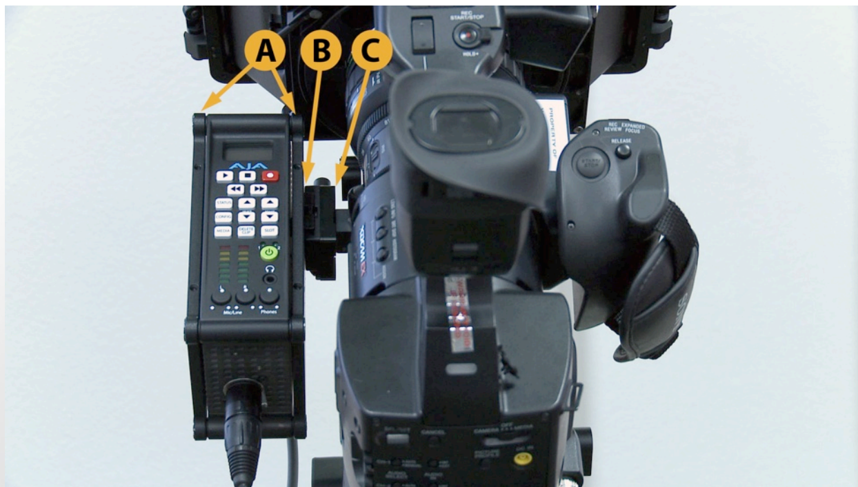
Example of Ki Pro Mini mounted to the side of the EX-1
