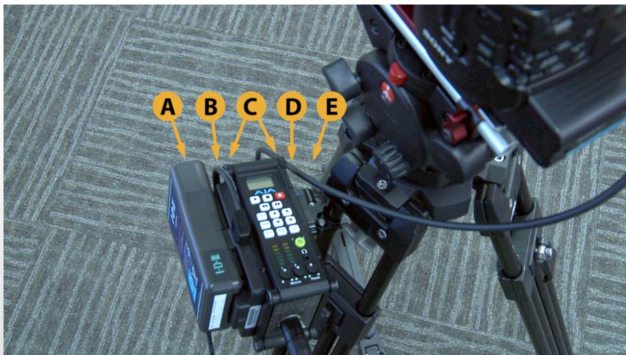
Example of Ki Pro Mini mounted to a tripod arm
