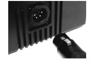
2. Insert into DC supply 3. Insert 4-pin XLR into 12Vdc Ki Pro power socket.
